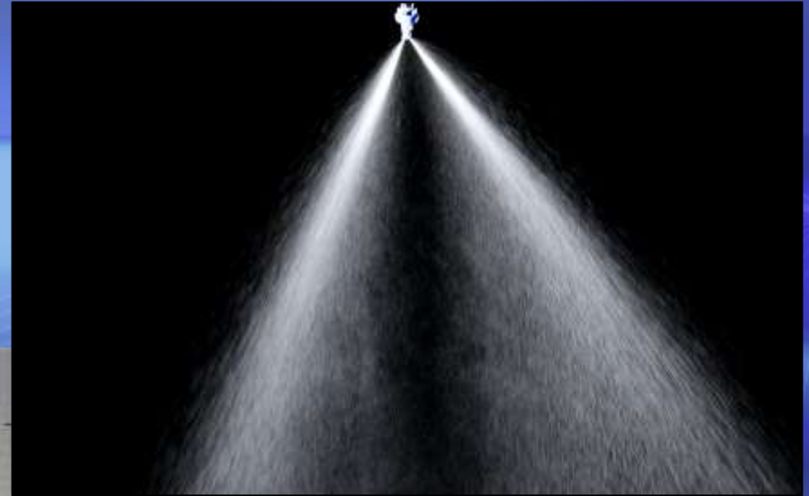
Spray video of the IDTA 120-03 at 5 bar.
